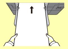
After printing starts, catch the paper when it is output so that it does not fall. When using the inner tray as the output location, do not stand up the stopper.
