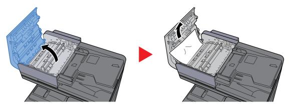
Turn dial (C) clockwise and remove any jammed originals.
