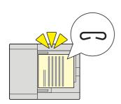
When reading a document from the document processor, if a stapled document is detected, then the reading stops automatically.
