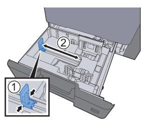
3 Adjust the position of the paper width guides located on the left and right sides of the cassette.
