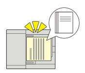
When reading a document from the document processor, if the multiple feeding of documents is detected, then the reading stops automatically.
