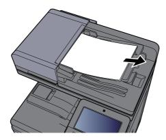
Open the front cover and remove any jammed paper.
