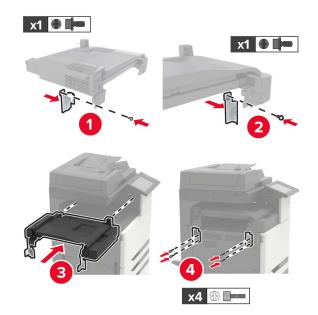
Attach the finisher to the printer.
