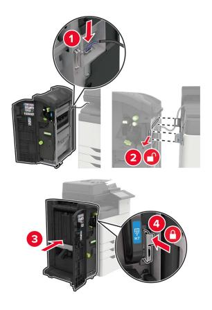
**9** Insert the staple cartridge into the finisher until it *clicks* into place.
