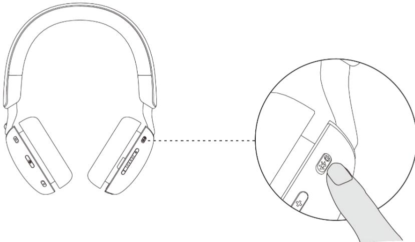
2. Press and hold the power button for 3 seconds, ensuring that the LED blinks blue, indicating the Bluetooth pairing has been initiated.
