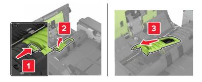
**4** Remove the ADF separator roller.
