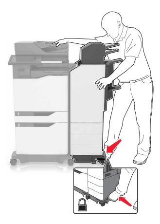
**15** Give the finisher a hard pull to check if it detaches from the printer. If the finisher detaches, then repeat <u>step 13</u> and <u>step 14</u> until they are properly locked.
