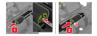
7 Insert the ADF separator roller cover until it *clicks* into place.
