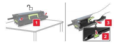
6 Unpack the new photoconductor unit, and then remove the packing material.
