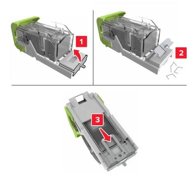
Note: Do not insert the staples that came out of the cartridge.
