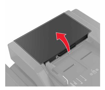
**3** Remove the ADF separator roller cover.
