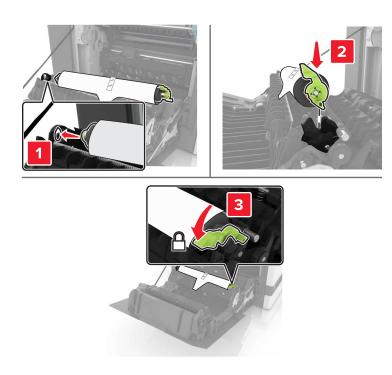
**5** Remove the white packing material.
