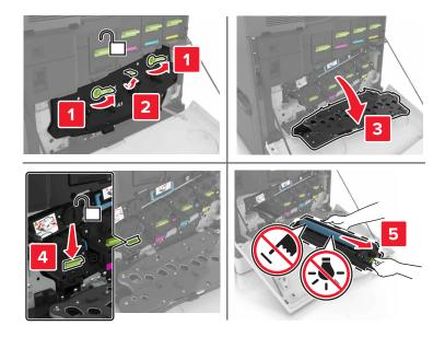
Remove the photoconductor unit.
