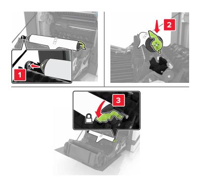
**5** Remove the white packing material.
