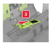
**4** Remove the ADF separator roller.
