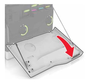
**3** Remove the keyboard attach cover.
