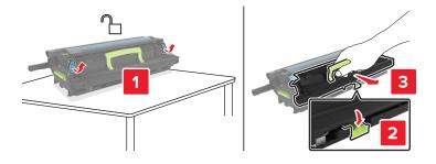
**5** Unpack the new developer unit, and then remove the packing material.
