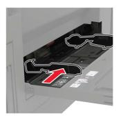
**3** Flex, fan, and align the paper edges before loading.
