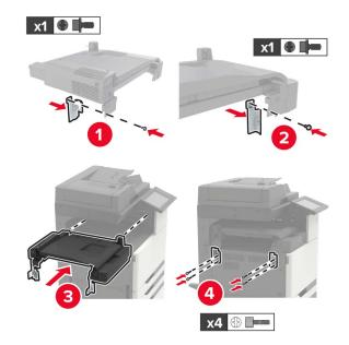
Attach the finisher to the printer.
