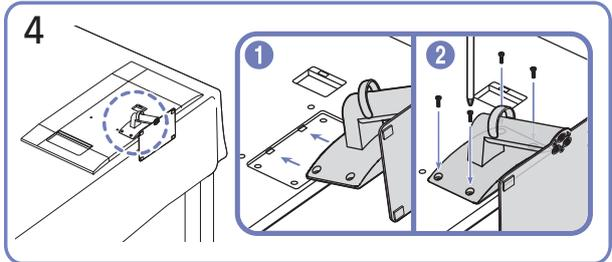
Push the assembled stand into the main body in the direction of the arrow as shown in the figure. Tightly fasten the connecting screw at the bottom of the main body.
