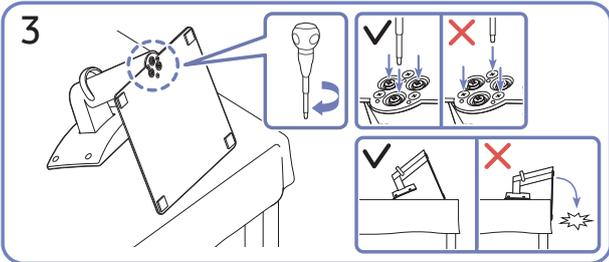
Place the stand on a table as shown in the figure. With the stand neck fastened vertically to the stand base, tightly fasten the connecting screws at the bottom of the stand base.
