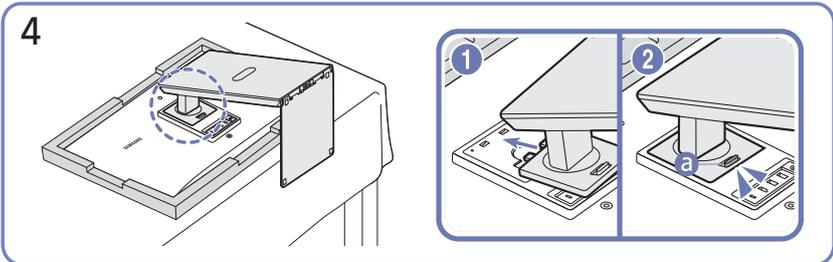
Push the assembled stand into the main body in the direction of the arrow as shown in the figure.
