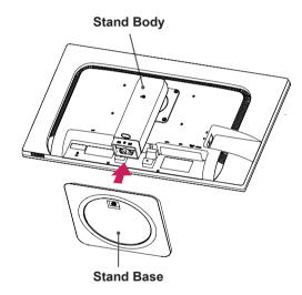
3 Using a coin, turn the screw clockwise to secure the **stand base**.
