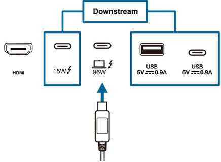
2. Uses HDMI port for video input, and Thunderbolt 4/USB type-c port for USB data input: Thunderbolt 4/USB-C input is upstream, and Thunderbolt 4/USB-C output/USB Type-C/USB Type-A are downstream.
