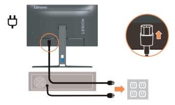
7. Connect the cables with cable clip.
