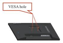
Step 5: Attach the LCD display to the wall, and follow the instructions in the wall-mounting kit. For use only with UL Listed Wall Mount Bracket with minimum weight/load: 8kg
