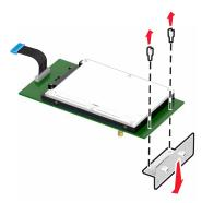
**7** Align the standoffs of the hard disk with the holes on the ISP, and then press the hard disk down until the standoffs *click* into place.
