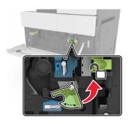
4 Remove the photoconductor unit.
