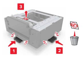
Remove the connector cover from the printer.
