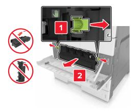
**3** Unlock the photoconductor unit.
