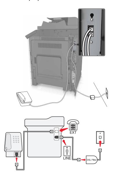
A Digital Subscriber Line splits your regular telephone line into two channels: voice and Internet. Telephone and fax signals travel through the voice channel, and Internet signals pass through the other channel. This way, you can use the same line for analog voice calls (including faxes) and digital Internet access.
