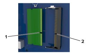
**4** Push the memory card straight into the connector, and then push the card toward the controller board wall until it *clicks* into place.
