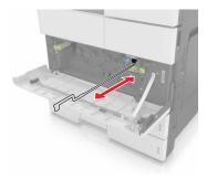
Remove the printhead wiper.
