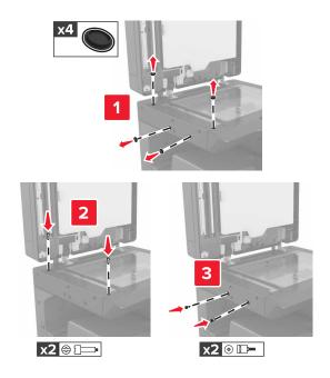
**Note:** Remove the screws after setting up the printer in another location.
