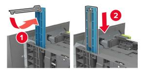
**d** Squeeze, and then slide the length guide to the correct position for the size of the paper being loaded.
