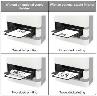
• When loading prepunched paper, make sure that the holes on the long edge of the paper are against the right side of the paper guide.
