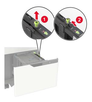
b If the A5 length guide is still attached, then remove it. If the guide is not attached, then proceed to <a href="step:10">step d on page</a>
