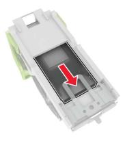
**Note:** If the staples are at the rear of the cartridge, then shake the cartridge downward to bring the staples near the metal bracket.
