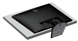
2. Use a screwdriver to press and hold the stand release button and then slide the stand assembly out of the monitor.
