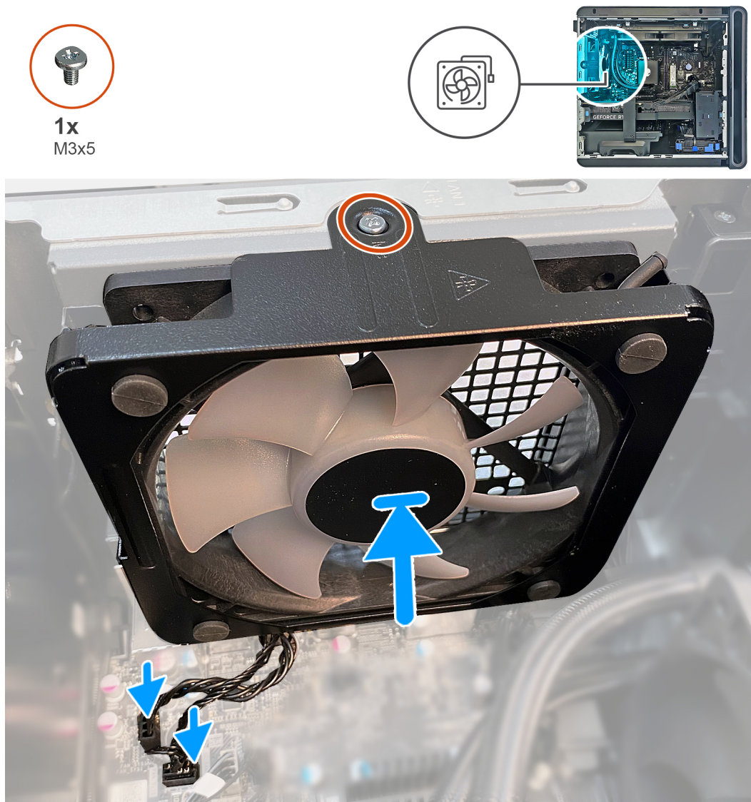
Figure 44. Installing the rear-chassis fan
