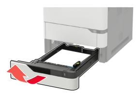
**Warning—Potential Damage:** A sensor inside the optional tray is easily damaged by static electricity. Touch a metal surface before removing the jammed paper in the tray.
