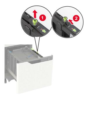
b If the A5 length guide is still attached, then remove it. If the guide is not attached, then proceed to <u>step d on page</u> <u>5</u>.
