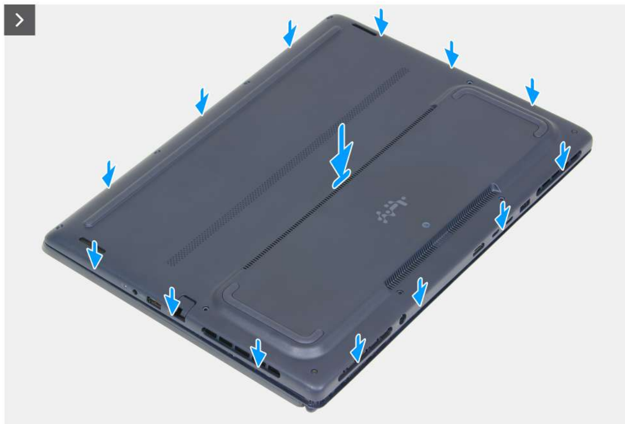
Figure 16. Installing the base cover
