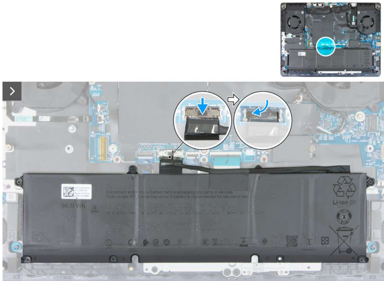
Figure 15. Connecting the battery cable
