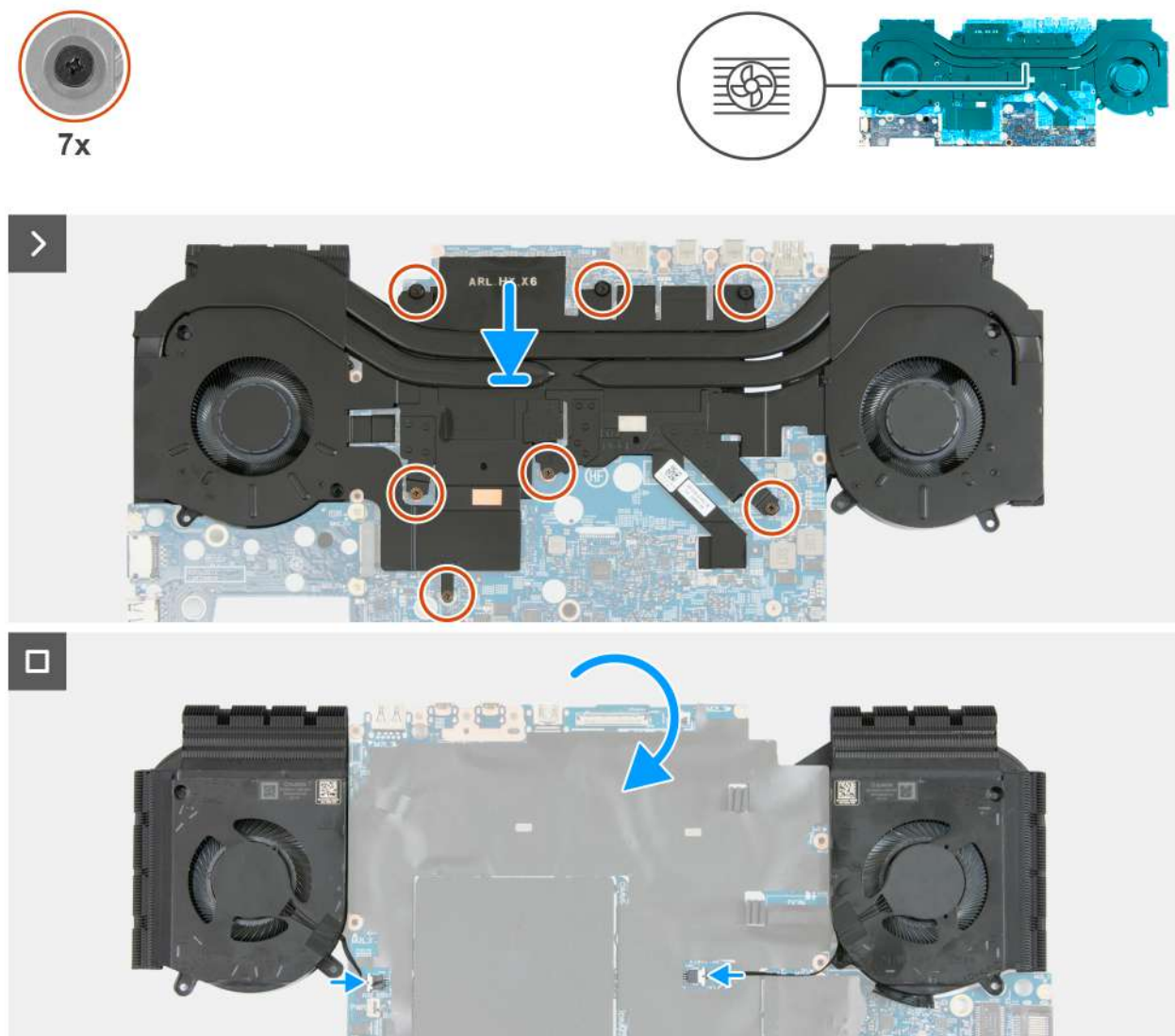
Figure 62. Installing the fan and heat-sink assembly
