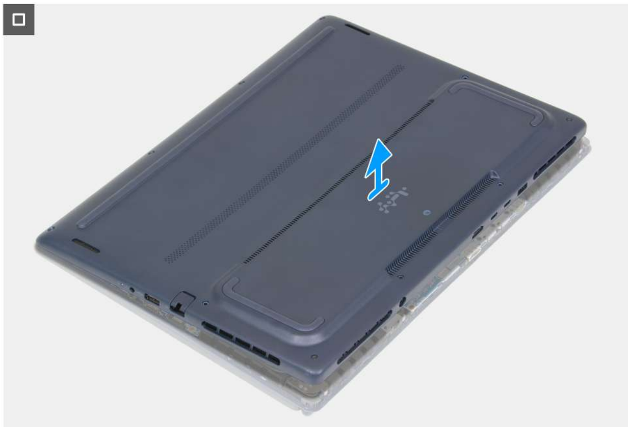
Figure 13. Removing the base cover
