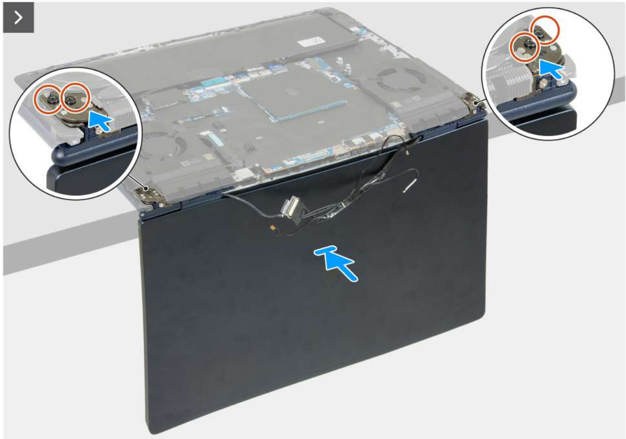
Figure 75. Installing the display assembly
