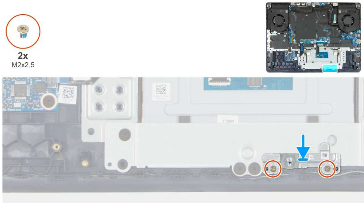
Figure 43. Installing the battery bracket
