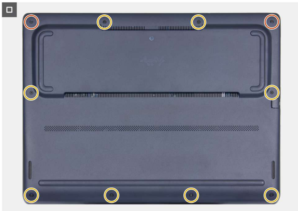
Figure 17. Installing the base cover
