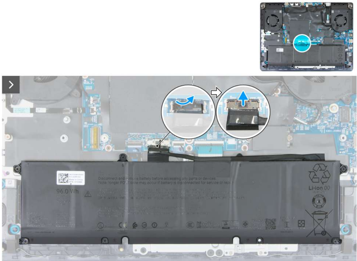
Figure 14. Disconnecting the battery cable
