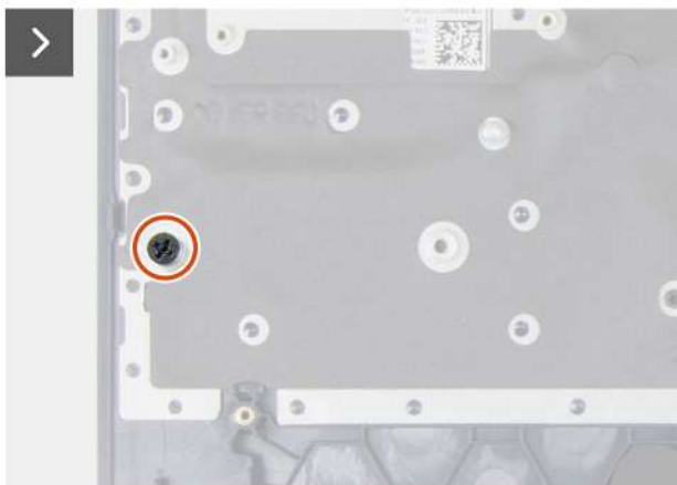
Figure 78. Removing SSD screw mounts
