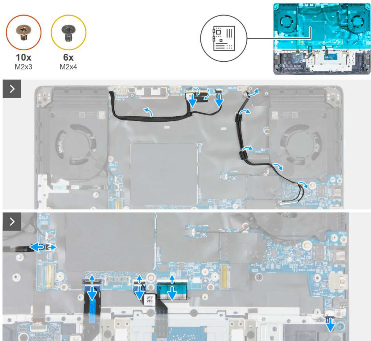
Figure 49. Removing the system board
