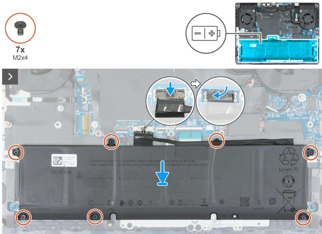
Figure 19. Installing the battery
