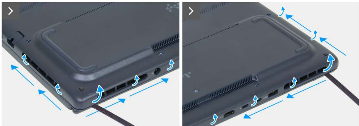
Figure 12. Inserting the scribe between the gap
