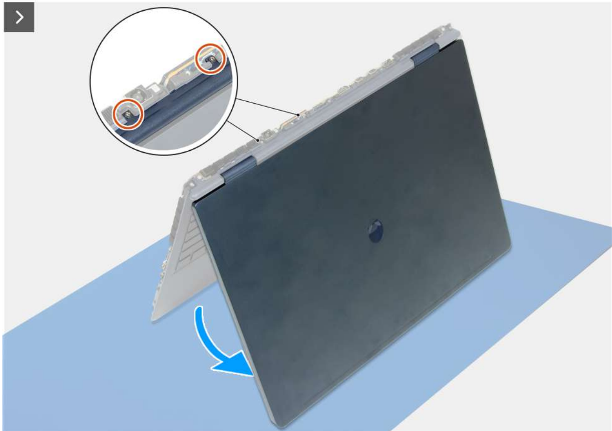
Figure 68. Removing the center bar
