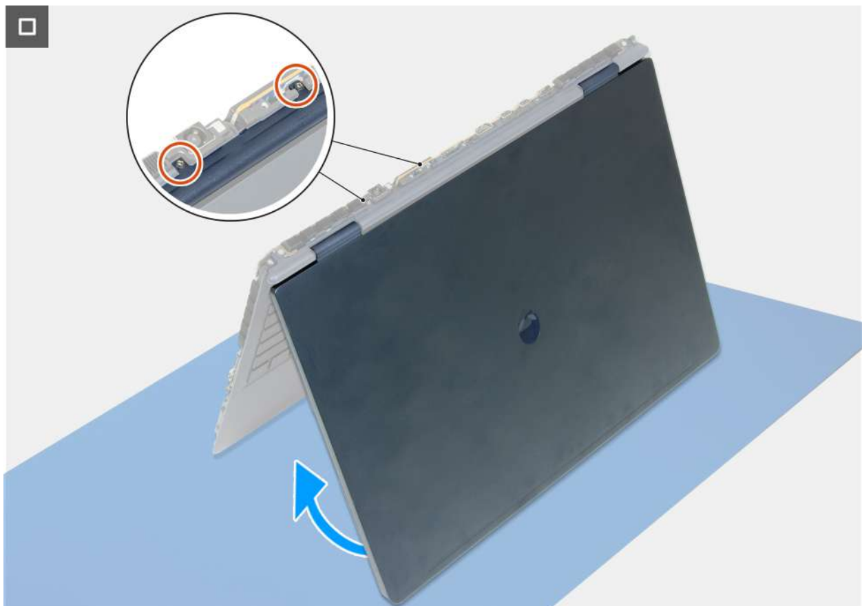
Figure 71. Installing the center bar
