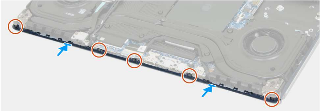
Figure 67. Installing the rear cap
