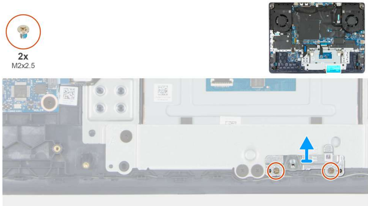
Figure 42. Removing the battery bracket
