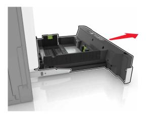
**2** Remove the separator bracket.
