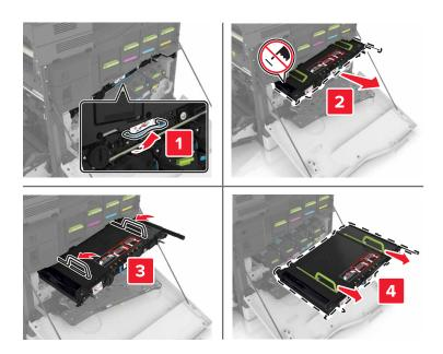
7 Unpack the new transfer belt, and then remove the packing material.
