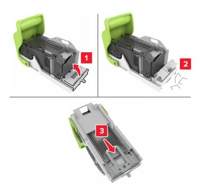
**Note:** Do not insert the staples that came out of the cartridge.
