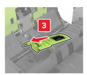
**4** Remove the ADF separator roller.
