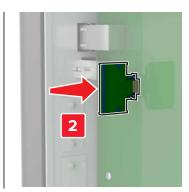
**Note:** The entire length of the connector on the card must touch and be flush against the controller board.
