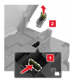
**4** Lift the staple guard, and then remove the loose staples.
