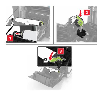
**5** Remove the white packing material.
