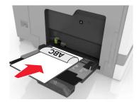
• Load envelopes with the flap side up and against the left side of the paper guide. Load European envelopes with the flap side up and entering the printer first.
