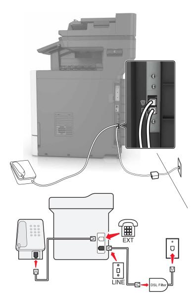
Digital subscriber line (DSL) splits your regular telephone line into two channels: voice and Internet. Telephone and fax signals travel through the voice channel, and internet signals pass through the other channel.
